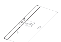
16 103.1901 Height: 2.0 mm knobs distance: 22.0 mm
