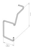
16 302.3201 Clamping spring for head box 55 x 50 mm; Shaft height 29.5 mm (2 pieces are required per drive)
